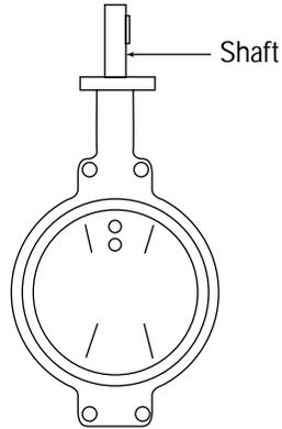
7. Insert taper pin(s) into the disc and set with two or three sharp blows. Wipe dust shield o-ring with silicone grease and place over the shaft into the top of the body.
