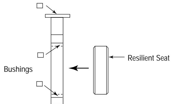
5. Completely coat the inside surfaces of the seat with silicone grease. Carefully push the disc into the seat in the open position (90 degrees to the body.) Line up the shaft holes of the disc as close as possible with the shaft holes in the seat body.
